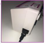
Run the mains cable through the cable management conduit, if applicable and plug into mains socket. Connect mains cable to pump.
