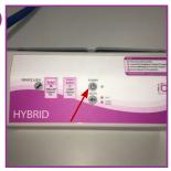
Switch the pump on via the POWER Button on Control Panel.
