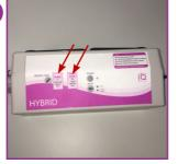
POWER LED will show green. If using CORE Hybrid, ensure CORE Hybrid FoC LED is flashing.
