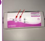
When correct pressure is reached, the SERVICE LOCK (either STELLAR or CORE) LED will stop flashing and remain constant. This signifies mattress has reached required pressure.
